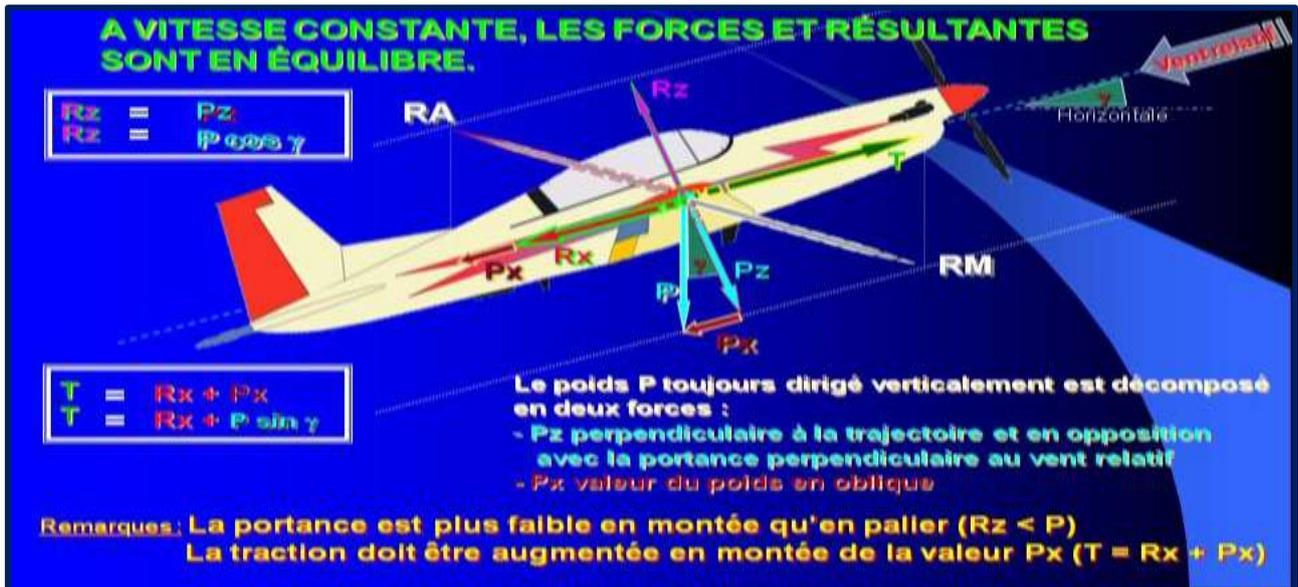
$$R_z = mg \cdot \cos \gamma \quad T = R_x + mg \cdot \sin \gamma$$
